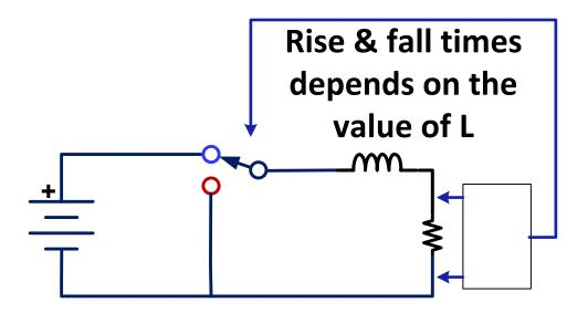
Effective value of L during 1-way (not full-cycle) operation depends on the winding of the inductor and to a small extent on the value of the magnetic field through it. The magnetic field is that of the earth.
